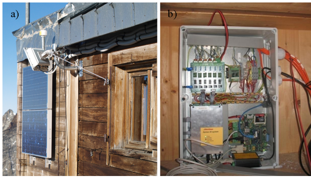
Fig. 3. (a) The solar panels, the GPS and the aerial radio installed outside the Carrel hut; (b) the acquisition system installed inside the hut (photo by Signori and Bani, 2010).
